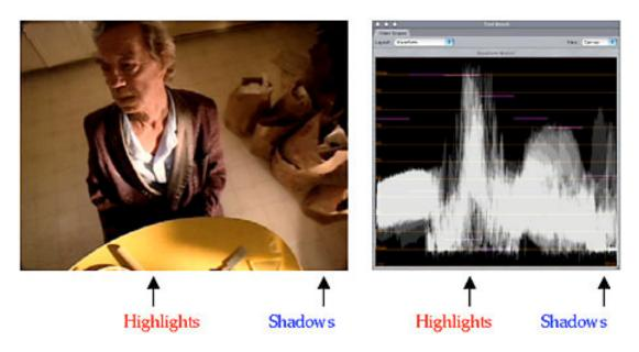
The image on the left is represented in the waveform monitor on the right. In order to understand it you must know a few things about waveform representations.
