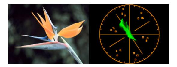
The flower has a particular shade of orange that can be clearly seen on the Vectorscope. If you needed to match that color to, say, some graphic then you could compare its Vectorscope reading and see the what the differences are. The other thing a Vectorscope is good for is confirming white balance. If you fill the frame with a white object then it should look something like this:
