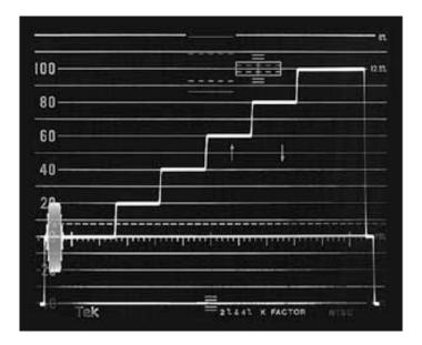
In this waveform we see a simple "staircase" test signal that has levels at 0, 20, 40, 60, 80, and 100 IRE from left to right. The step on the left would be below black, the next step a dark gray, the next step a bit lighter gray and so on up to the last step which would be bright white. It looks like this:
